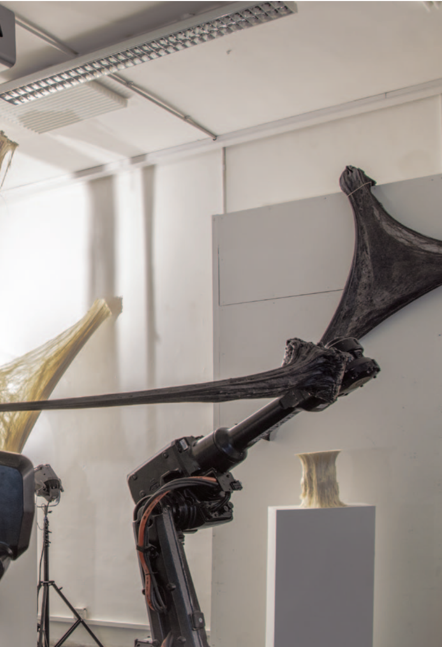
30 The ABB IRB2600 MultiMove system of three six-axis industrial robots, stretching soft foam (REX | LAB, installed at Smartgeometry 2013)
